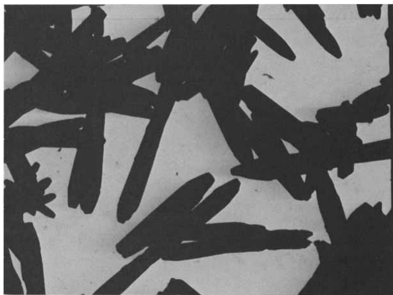
FIG. 3f. Microphotograph of the precipitate: \bar{d}_p = 2.11 \mu\text{m} , \text{pH} = 9 , t = 98^\circ\text{C} , and indirect method.
