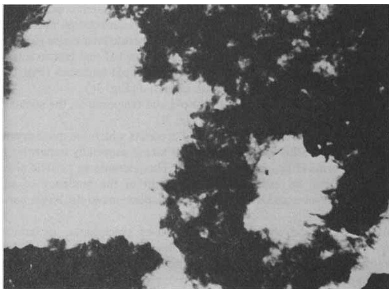
FIG. 3b. Microphotograph of the precipitate: \bar{d}_p < 0.10 \mu\text{m} , \text{pH} = 10 , t = 25^\circ\text{C} , and direct method.
